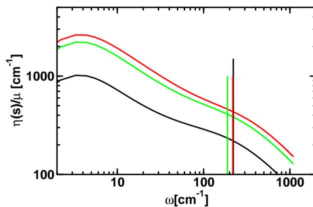
Figure 4: Laplace transform of friction for DFT (black), OPLS (red), and DANG-SPC/E (green). Impulse lines indicate the barrier frequency for each of the cases.
