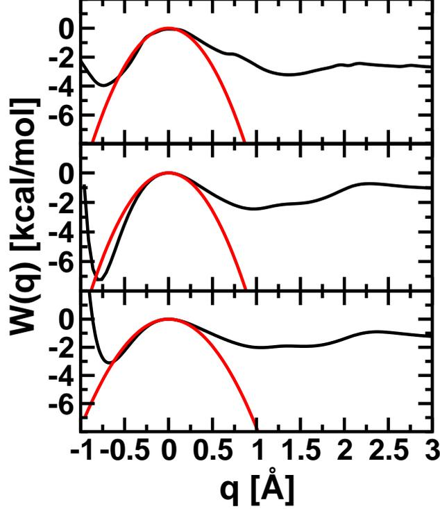
Figure 1: The Potential of mean force (black) and the harmonic fit to the transition state region (red) for DFT, OPLS-TIP4P and DANG-SPC/E from top to bottom.
